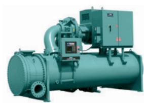
YK Water to water heat pump VSD Centrifugal compressor / R1234ze Hot water up to 68°C Hot water up to 93°C (High Pressure casing only) Heating capacity: 1000 to 9000 kW
