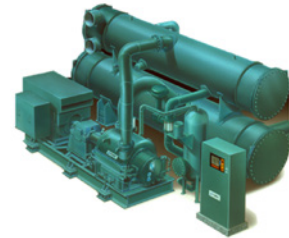
Titan OM HP Water to water heat pump Multi-stage Centrifugal, electric, steam or gas driven / R1234ze Hot water up to 95°C Heating capacity: 5000 to 20000 kW
