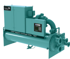
YMC 2 Water to water HP VSD Centrifugal Magnetic bearings R513A Hot water up to 65°C Heating capacity: 1600 to 3000 kW
